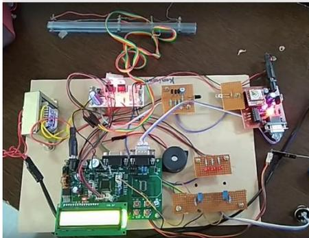
Fig.10. System design model of GPRS based smart water quality monitoring system
