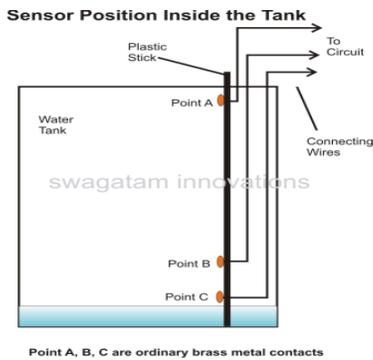
Fig.7. Water Level Sensor
