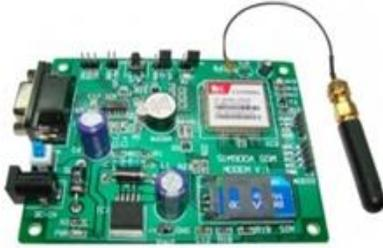
Fig 3. GPRS modem
