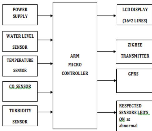
Fig.2. Block Diagram of Smart Water Quality Monitoring System
