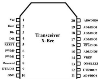
Fig 4. ZIGBEE pin diagram
