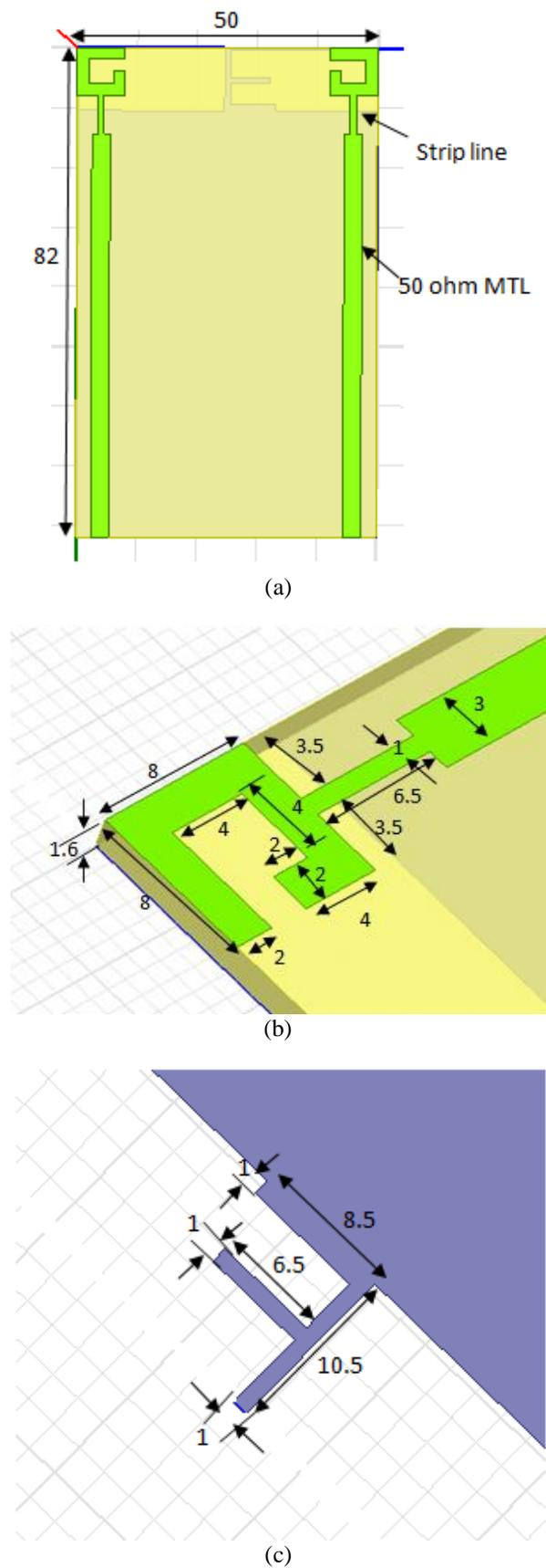
Fig. 1. 3D structure of MIMO antenna (a) overall view, (b) detailed view of G shape antenna (c) detailed view of isolation. (dimensions are in mm)
