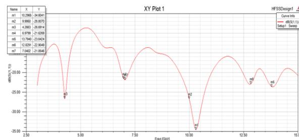
Fig. 5. Simulated return loss S11 versus frequency
