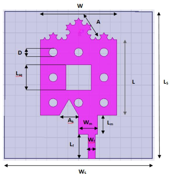
Fig. 4. Geometry of the proposed antenna.
