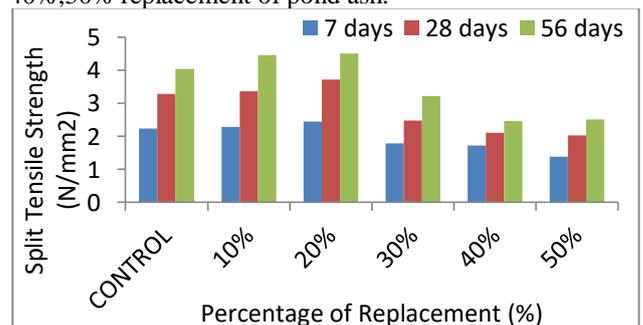
Fig. 3 Split tensile strength of concrete at various replacements at 7, 28 and 56 days
