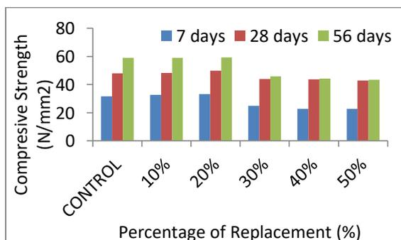
Fig. 2 Compressive strength at various percentage replacements at 7, 28 and 56 days.
