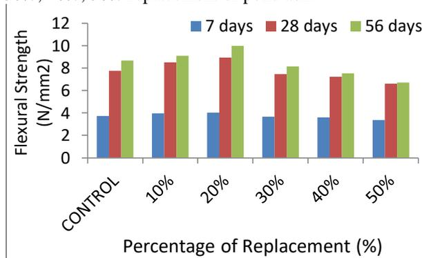
Fig. 4 Flexural strength at various percentage replacements at 7, 28 and 56 days
