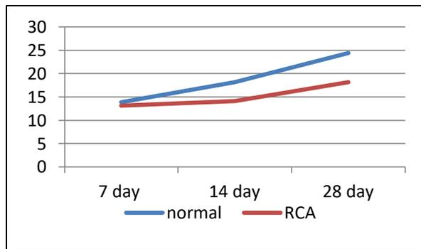
Fig 7. Reduction in Compressive Strength.
