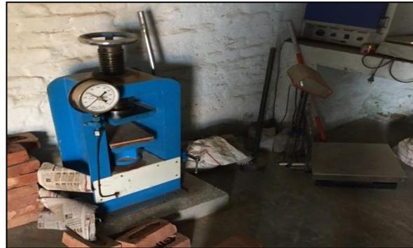
Fig 5. Compressive Strength Testing Machine.
