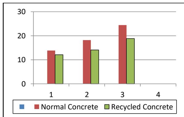
Fig 6. Compressive strength of Normal & RCA concrete.
