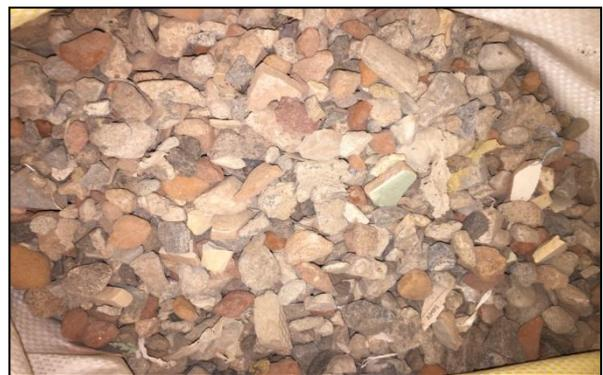
Fig 3. Recycled Coarse Aggregate.
