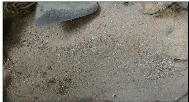
Fig 2. Recycled Fine Aggregate.
