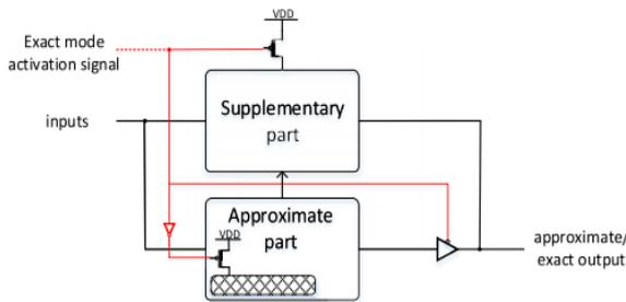
Fig .3. Block diagram of the proposed approximate 4:2 compressors
