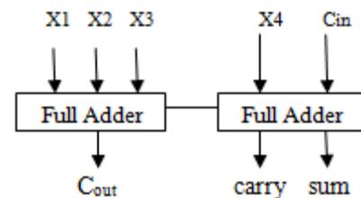
Fig. 2. Structure of the conventional 4:2 compressor
