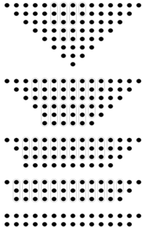
Fig. 7. Reduction circuitry of an 8-bit Dadda multiplier.
