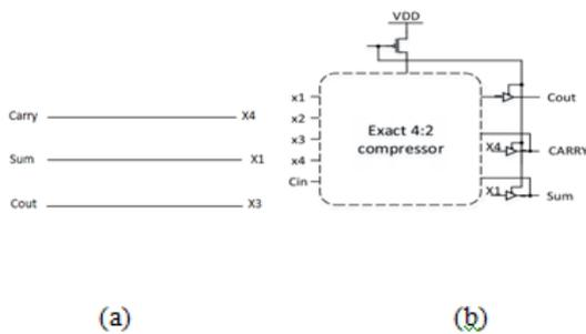
Fig.5. (a) Approximate part structure of DQ 4:2C2
