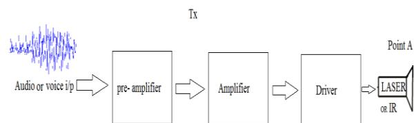
Fig.1. Transmitter section of LASER Communication
