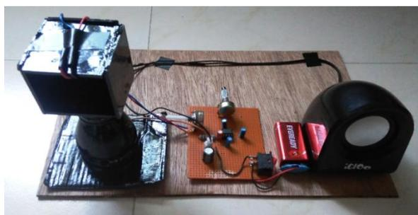
Fig. 9(b) Hardware implementation of Receiver
