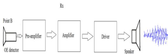
Fig.2. Receiver section of LASER Communication
