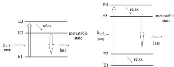
Fig. 5 Three and four level atomic system
