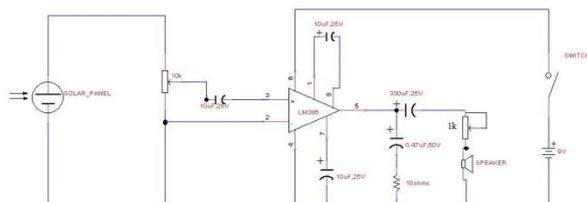
Fig. 9(a) Circuit diagram of Receiver
