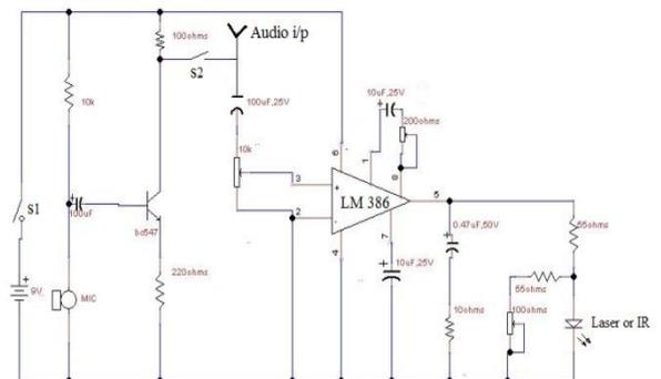
Fig. 8 (a) Circuit diagram of transmitter
