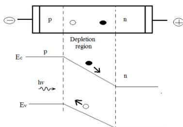
Fig.6. P-N junction energy band diagram showing carrier generation and their drift
