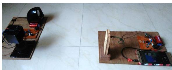
Fig. 10. Transmission and Receiver with line of sight alignment
