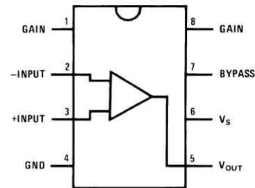
Fig. 7. Pin out configuration of LM386
