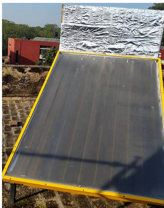
Fig. 2(b) Actual picture of flat plate collector with reflector attached on top (upper) side at an angle of 135 degree to the collector top surface.
