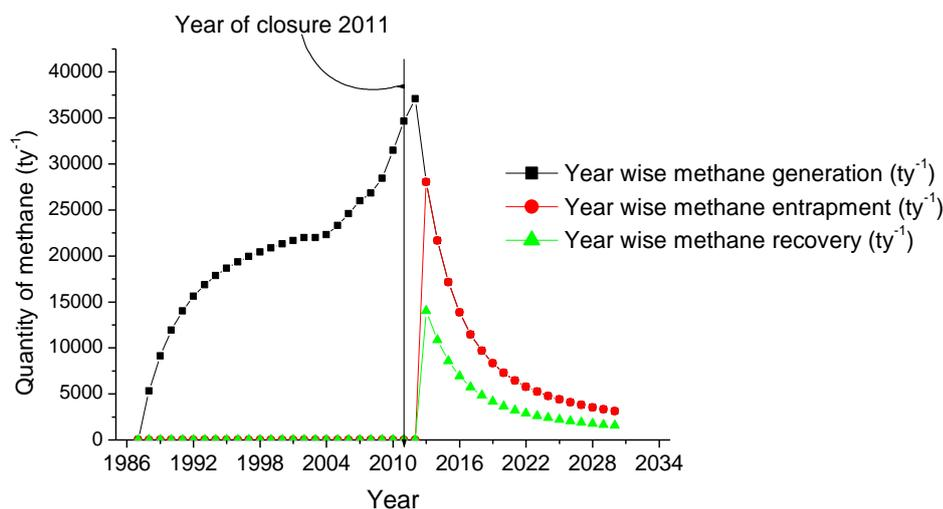
Fig. 3. Year wise methane generation, entrapment and recovery from existing open dump site following IPCC method
