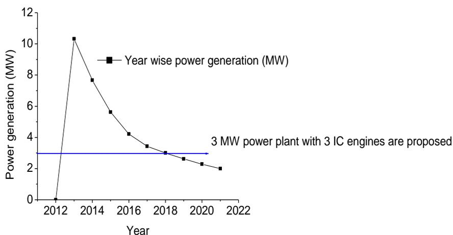
Fig. 5. Proposed power generation from existing open dump site, Dhapa
