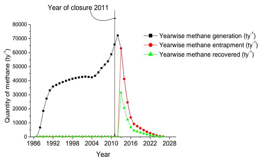
Fig. 2. Year wise methane generation, entrapment and recovery from existing Dhapa landfill site following Triangular model
