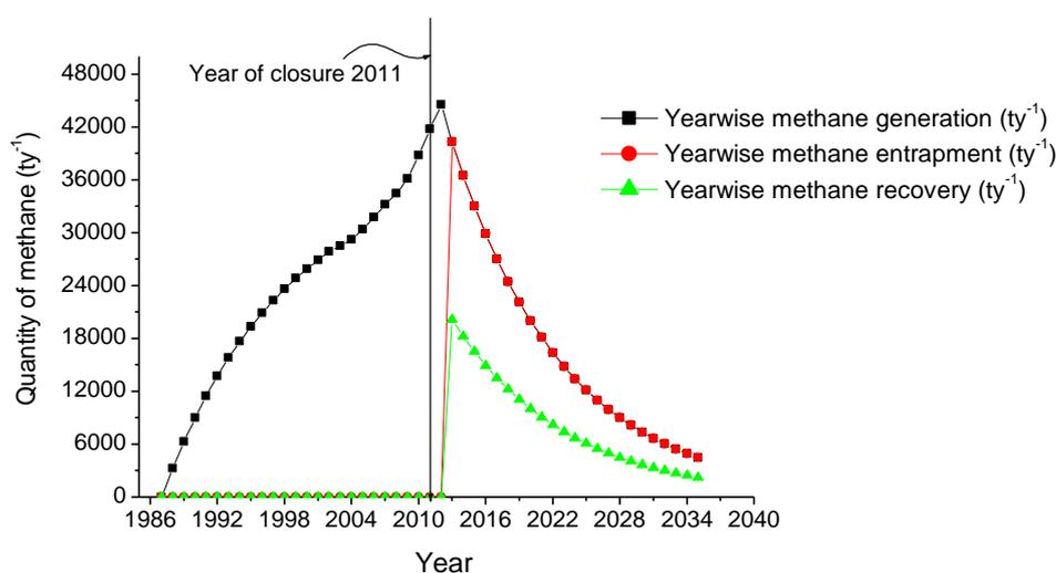
Fig. 4. Year wise methane generation, entrapment and recovery from open dump site Dhapa following LandGEM method
