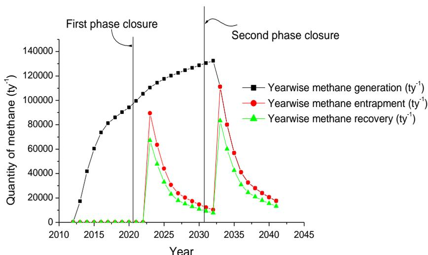
Fig. 6. Year wise generation, entrapment and recovery of methane from proposed engineered landfill site
