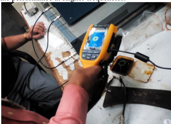
Fig. 11. Measurement of the temperature using FLIR IR camera
