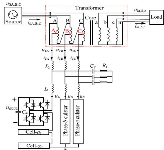
Fig.3.1. simulation model circuit.
