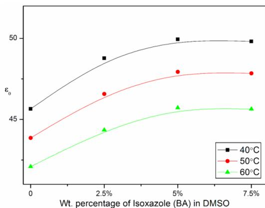
**Fig.6** Static dielectric permittivity ( $\epsilon_0$ ) for BA-DMSO at different temperatures.
