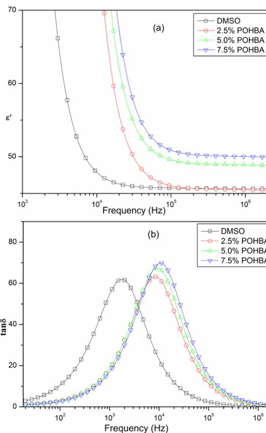
**Fig. 5** a) shows the frequency dependent spectra of the real part of the relative dielectric function  $\epsilon'$  and b) dielectric loss tangent,  $\tan\delta$  of POHBA-DMSO binary mixtures.
