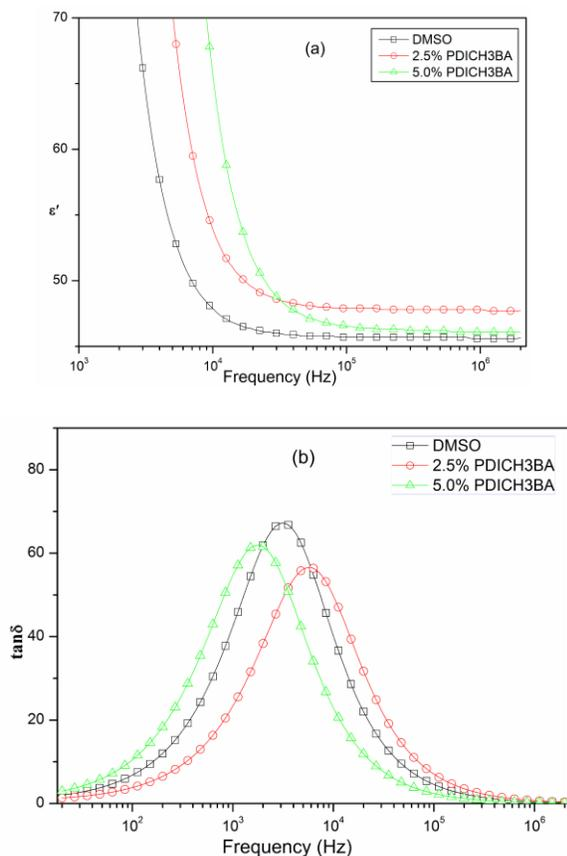
**Fig.3** a) shows the frequency dependent spectra of the real part of the relative dielectric function  $\epsilon'$  and b) dielectric loss tangent,  $\tan\delta$  of PDICH3BA-DMSO binary mixtures.
