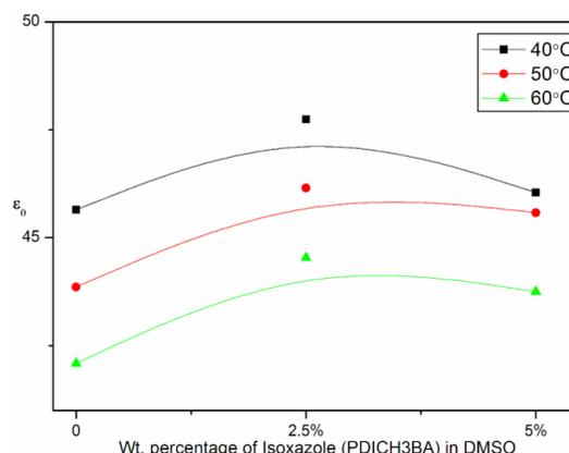
**Fig.7** Static dielectric permittivity ( $\epsilon_0$ ) for PDICH3BA-DMSO at different temperatures.
