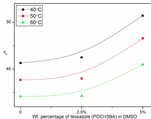
**Fig.8** Static dielectric permittivity ( $\epsilon_0$ ) for POCH3BA-DMSO at different temperatures.
