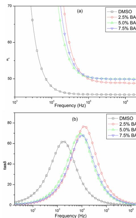
Fig. 2 a) shows the frequency dependent spectra of the real part of the relative dielectric function  $\epsilon'$  and b) dielectric loss tangent,  $\tan \delta$  of BA-DMSO binary mixtures.
