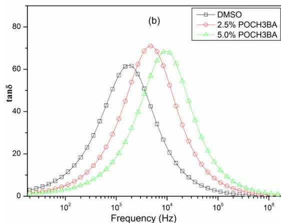
**Fig. 4** a) shows the frequency dependent spectra of the real part of the relative dielectric function  $\epsilon'$  and b) dielectric loss tangent,  $\tan\delta$  of POCH3BA-DMSO binary mixtures.
