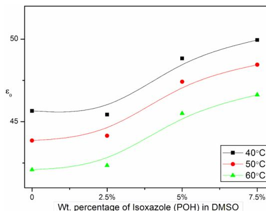
**Fig.9** Static dielectric permittivity ( $\epsilon_0$ ) for POHBA-DMSO at different temperatures.
