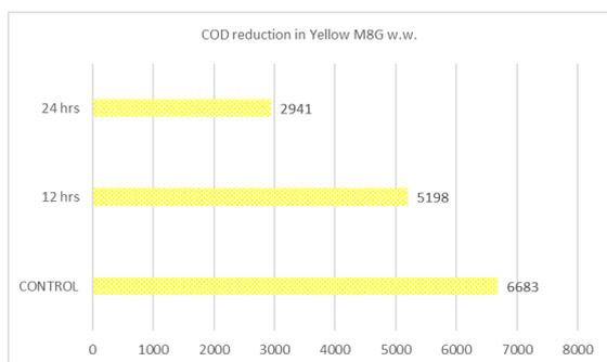
Fig:2 COD value of Yellow M8G waste water for control, 12 hrs and 24 hrs
