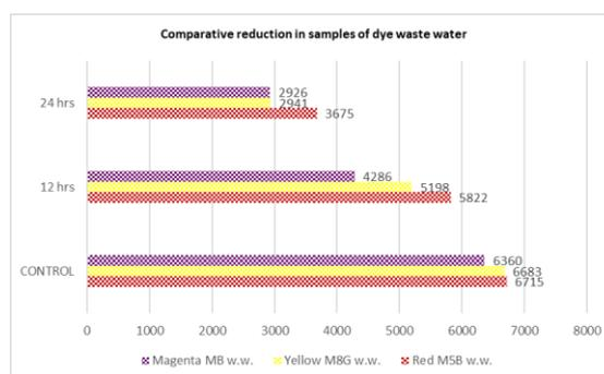
Fig:4 COD values of all three samples for control, 12 hrs and 24 hrs
