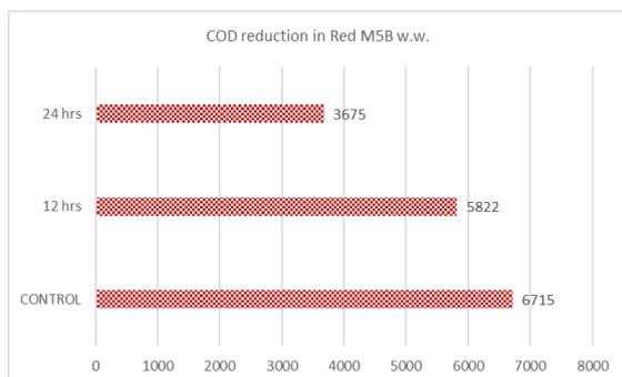
Fig:3 COD values of Red M5B waste water for control, 12 hrs and 24 hrs
