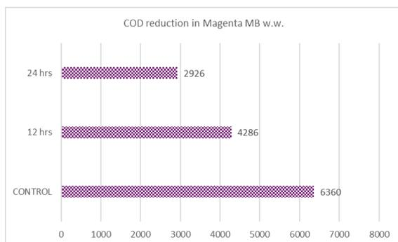
Fig:1 COD value of Magenta MB waste water for control, 12 hrs and 24 hrs
