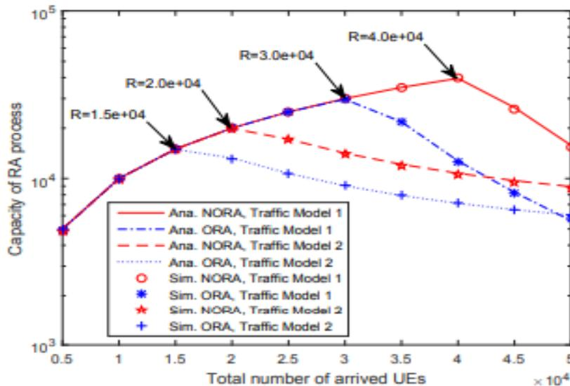
Fig. 2. Throughput Of RA process of the NORA and ORA schemes under both Traffic Models.
