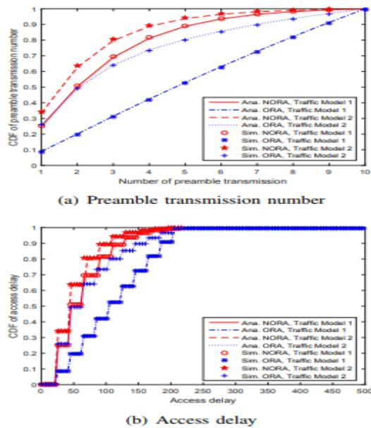
Fig. 4. CDF of the number of preamble transmissions and access delay for the successfully accessed UEs in NORA and ORA schemes under both Traffic Models.
