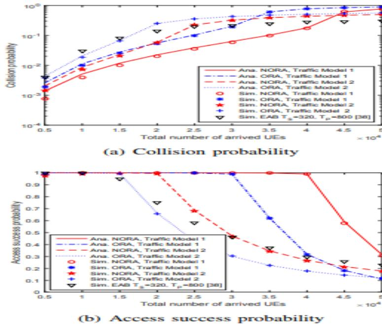
Fig. 3. Collision and access success probability of the NORA and ORA schemes under both Traffic Models.
