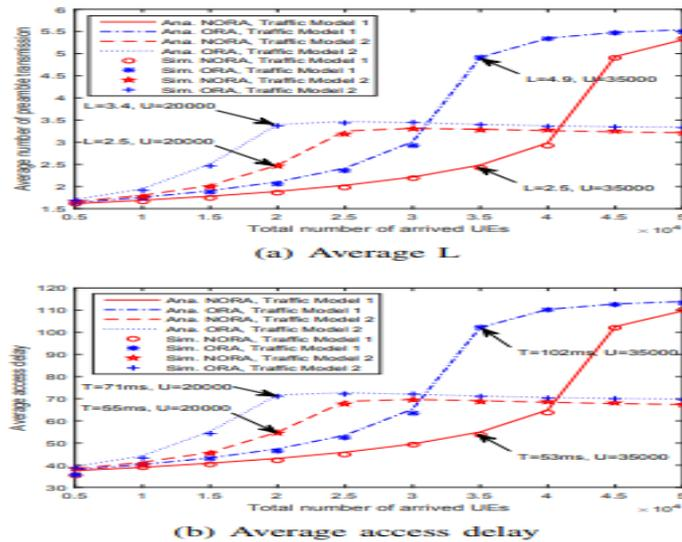
Fig. 5. Average number of preamble transmissions and access delay for the successfully accessed UEs in NORA and ORA schemes under both Traffic Models.
