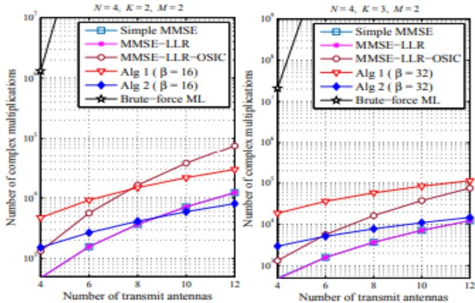
Fig. 5. Complexity comparison of different detection algorithms for MIMOOFDM-IM with  $N = 4,$  and BPSK modulation.
