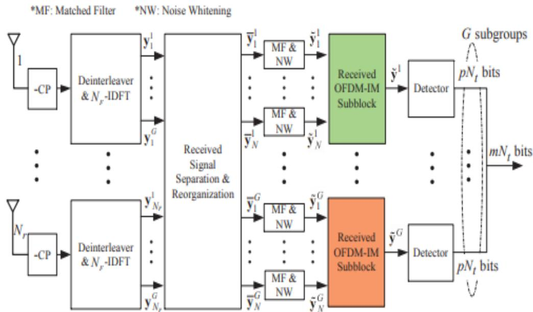
Fig. 2. Block diagram of MIMO-OFDM-IM receiver.
