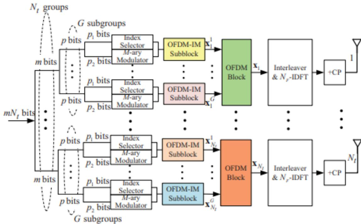
Fig. 1. Block diagram of MIMO-OFDM-IM transmitter.
