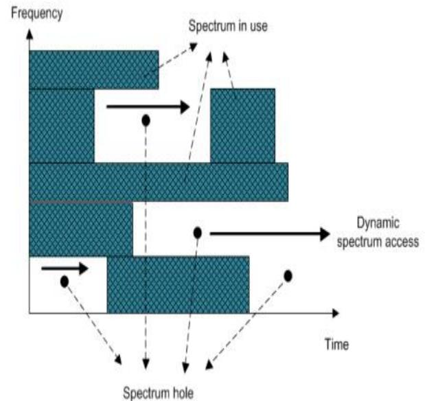
Figure 1: Spectrum hole and dynamic spectrum access.
