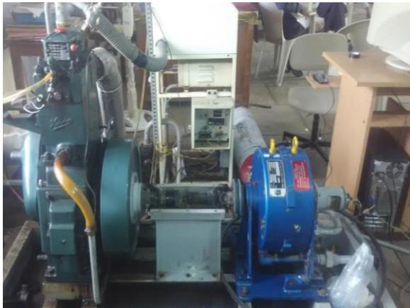
Figure 1: Single cylinder 4-stroke diesel engine test rig
