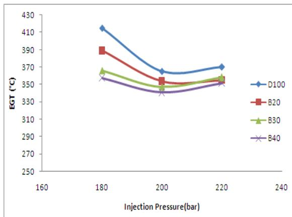
Figure 4: Influence of injection pressure on exhaust gas temperature
