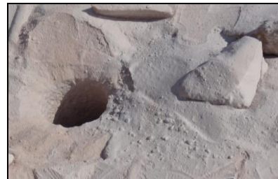
Figure 2 Filed Photo of Blast holes
