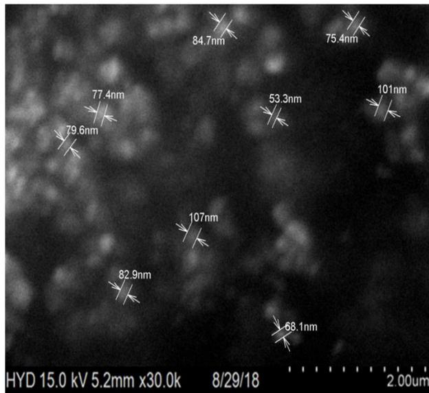
Fig. 3.1(c): SEM image for Nickel Nanoparticles (0.05 M Nickel chloride solution)
