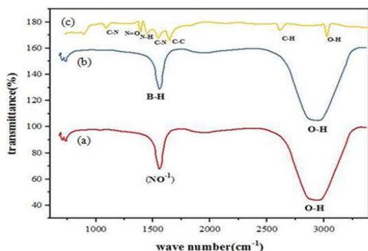
Fig. 3.3(2): FT-IR spectrum of Ni nanoparticles (a). 0.01 M (b). 0.05 M (c). Chemical Reduction Method
