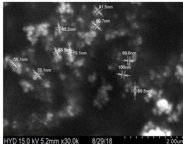
Fig. 3.1(a): SEM image for Nickel Nanoparticles (0.01 M Nickel chloride solution)
