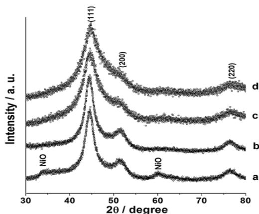
Fig. 3.2: XRD pattern of Nickel nanoparticles (a). Chemical Reduction Method (0.05 M) (b). 0.1 M (c). 0.05 M (d). 0.01 M
