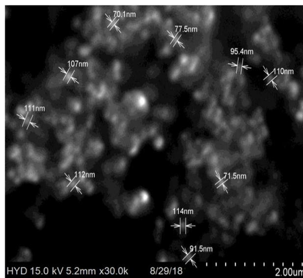
Fig. 3.1(b): SEM image for Nickel Nanoparticles (0.1 M Nickel chloride solution)
