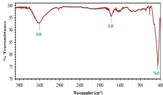
Fig. 3.3(1): FT-IR spectrum of 0.1 M Ni nanoparticles
