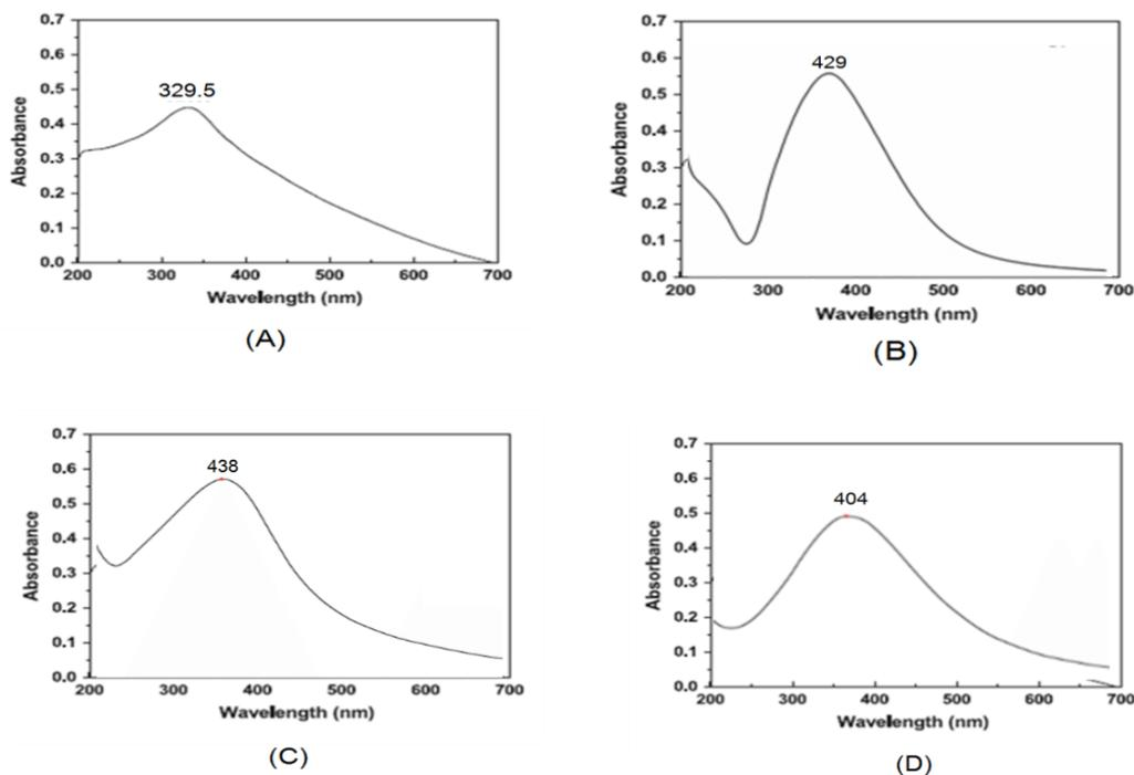
Fig. 3.4: UV-Vis spectrum of Ni nanoparticles (A) 0.1 M (B). 0.05 M (C). 0.01 M (D). Chemical Reduction Method
