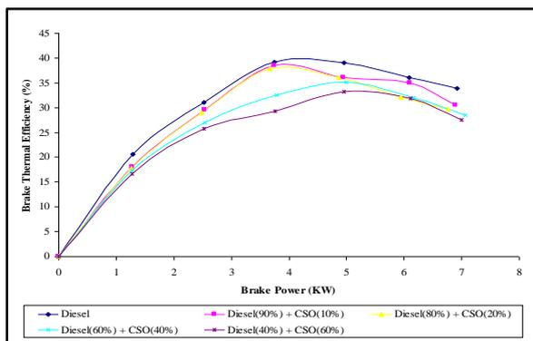
Fig.4. Brake power (kW) Vs Brake thermal efficiency(%)
