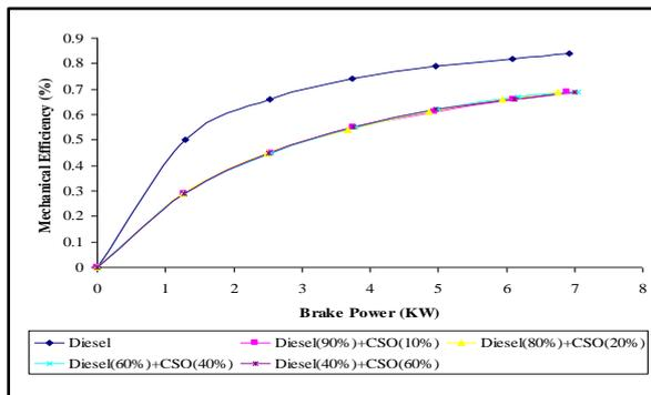
Fig.3. Brake power(kW) Vs Mechanical effi.(%)
