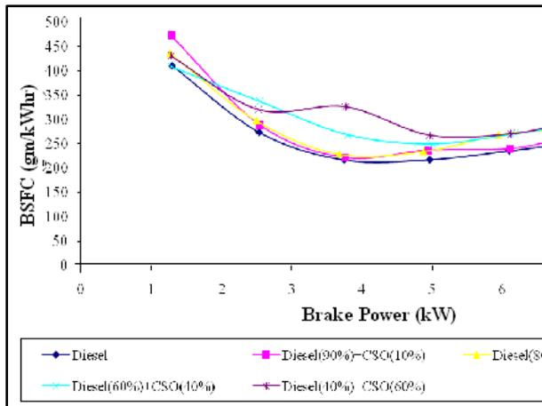
Fig.2. Brake power(kW) Vs BSFC(gm/kWhr)
