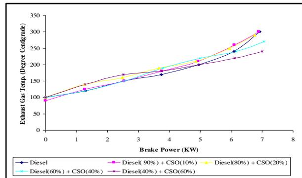
Fig.5. Brake power (kW) Vs Exhaust gas temperature (°C).
