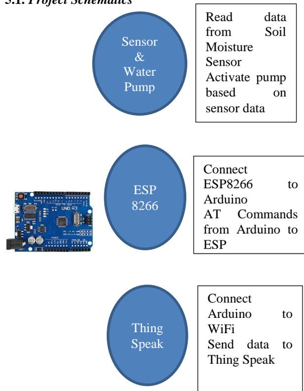
Arduino Uno is the core embedded system of this project. This Arduino Uno acts as the central driving system of the project and has to be interfaced with three different components of the system namely the Soil moisture sensor and water pump, ESP 8266 and ThingSpeak API.
