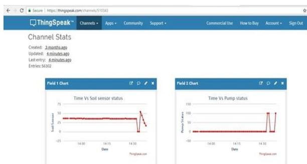
Fig 4. Thingspeak graph when moisture level drops
