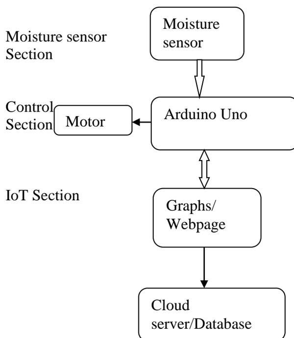
Fig. 1. Smart Irrigation System Using IoT – Block Diagram
