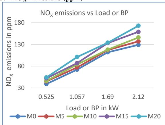
Fig.9 Variation of NO<sub>x</sub> Emission with Engine Load
