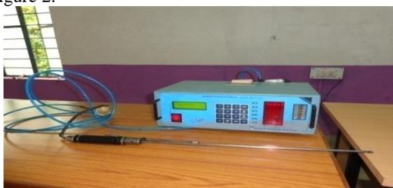
Fig.2 Exhaust Gas Analyser
