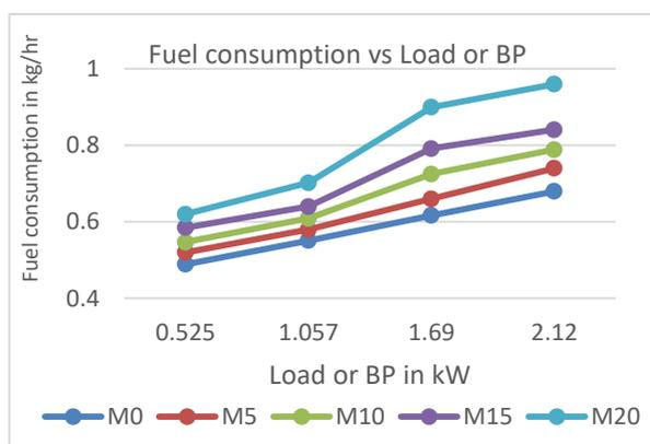
Fig.3 Variation of Fuel consumption with Engine Load
