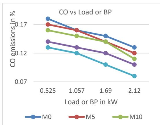
Fig.6 Variation of CO Emission with Engine Load
