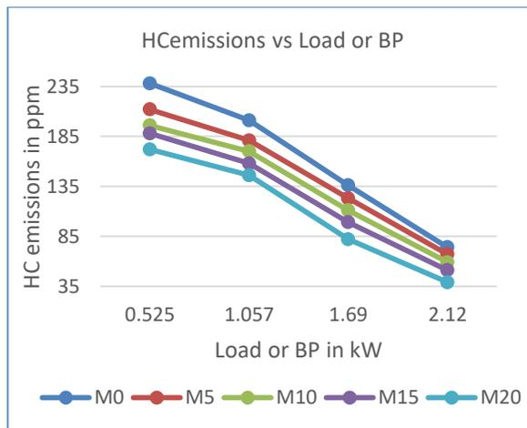
Fig.7 Variation of HC Emission with Engine Load
