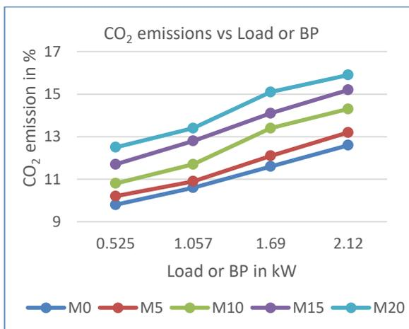
Fig.8 Variation of CO<sub>2</sub> Emission with Engine Load
