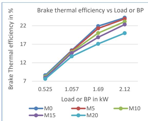
Fig.5 Variation of Brake Thermal Efficiency with Engine Load
