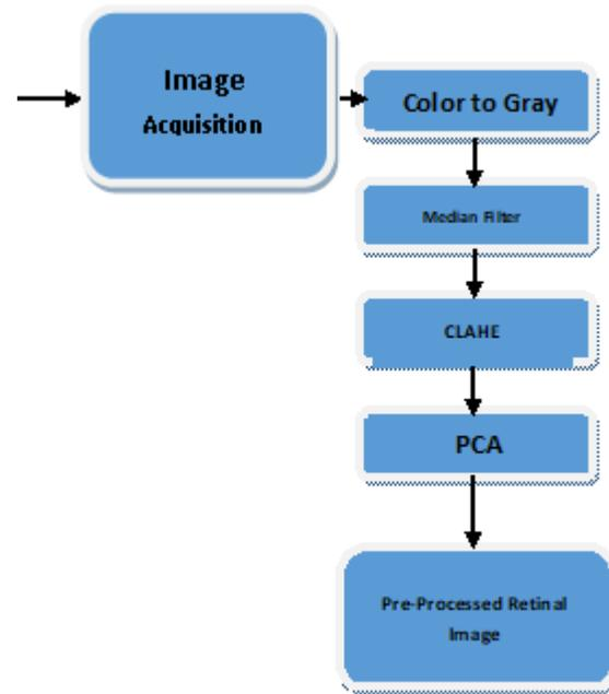
Figure 7. Block Diagram of the Proposed Pre-Processing Technique.
