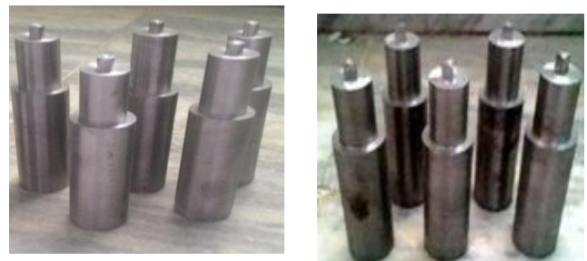
Fig. 2: Cylindrical, square and triangular FSW tools
