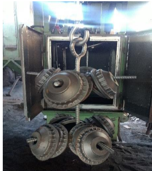
Fig.1. Existing Hanger with casting
