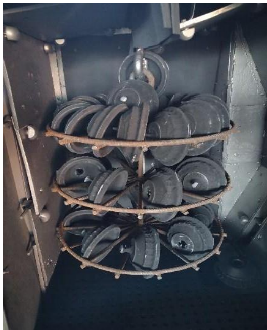
Fig.7. Hanger with Casting before Shot Blasting
