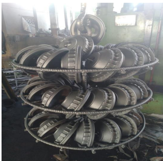
Fig.8. Hangers with Casting after Shot Blasting
