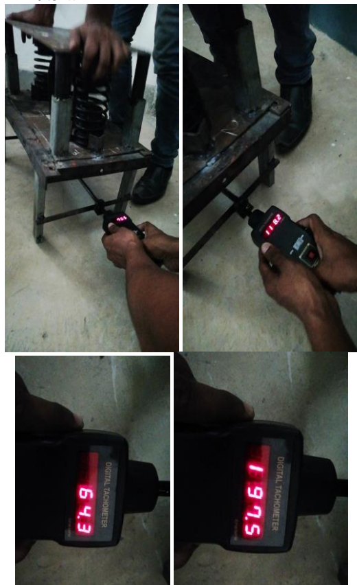
Fig. 5. Speed measuring with Tachometer
