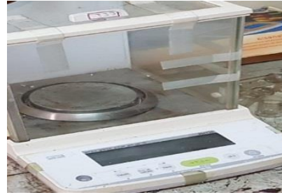
Fig 6. Weight of tool and work piece was measured using SHIMADZU ATY224
