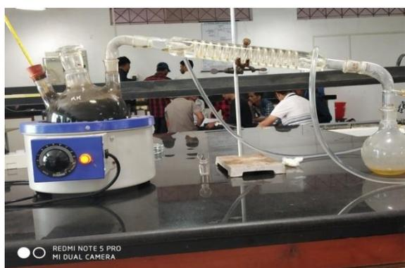
Fig 2: Vacuum Distillation Unit
