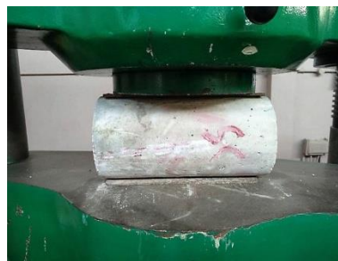
Pic 5-Split tensile Test
