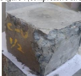
Pic 3- Cube after failure
