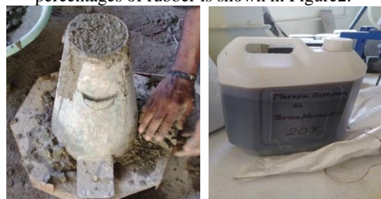
Pic 2 Slump test and glemium
