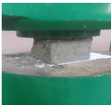
Pic 4-Compression Test
