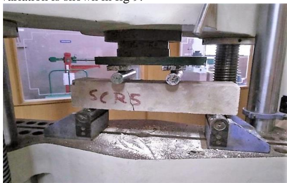
Pic 6-Flexural Test
