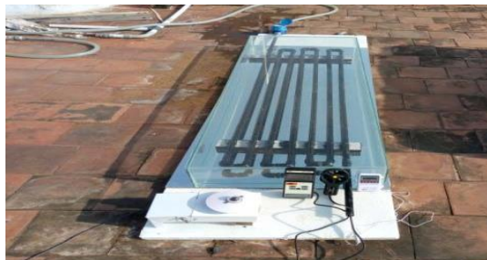
Fig.1.1 Side view of the multiple pipe line solar instant water heater using reflecting mirror.
