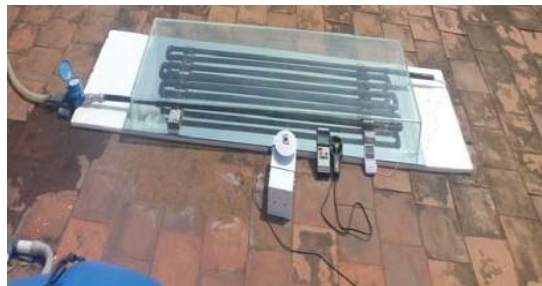
Fig.1.2 Top view of multiple pipes solar instant water heater using a ready reflecting mirror.
