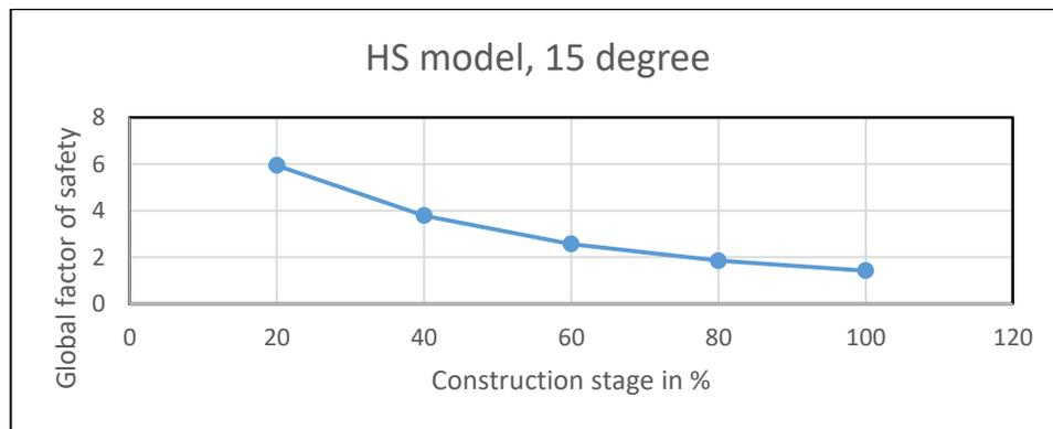
Figure 4: FOS with construction stages
