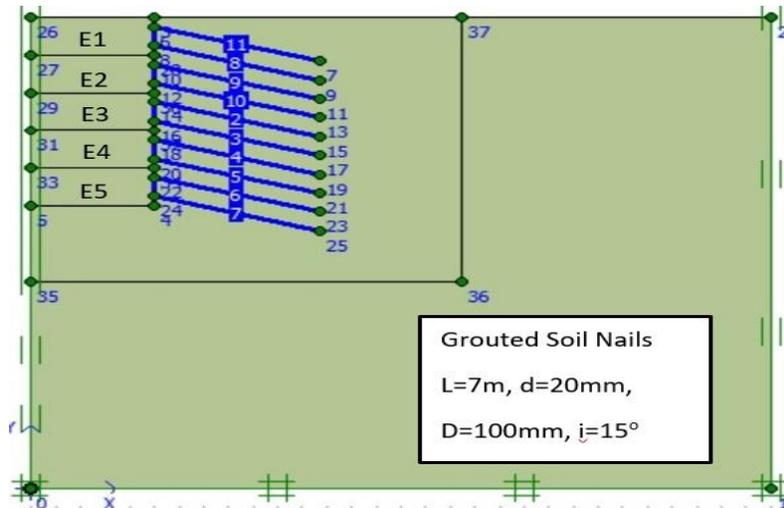
Figure 2: The Simulation model of soil nail wall with a 15-degree inclination and nail length-7m
