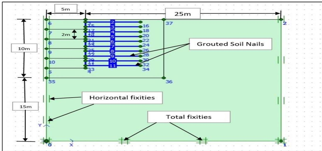
Figure 1: FEM soil nail wall with no inclination, 10m high
