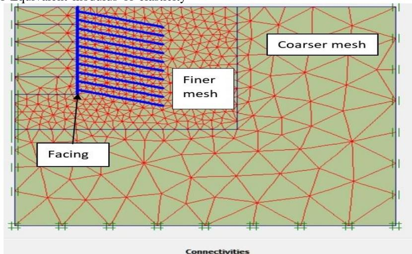
Figure 3: Simulated soil nail wall with different clustered mesh generation
