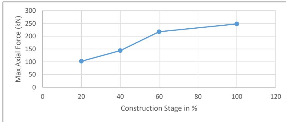
Figure 7: Development of Axial Force in soil nails
