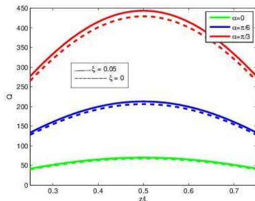
**Fig.4 :** Variation of volumetric flow rate  $Q$  with  $z/L$
