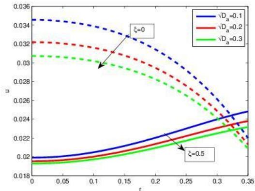
**Fig.3 :** Variation of axial velocity  $u$  with radius  $r$  for different values of Darcy number  $\sqrt{D_a}$ .
