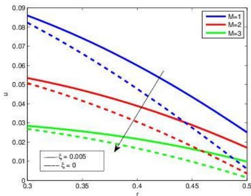
**Fig.2 :** Variation of axial velocity  $u$  with radius  $r$  for different values of Magnetic field  $M$ .
