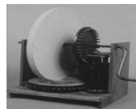
Fig. 1. 1st Polishing machine by Leonardo da Vinci
