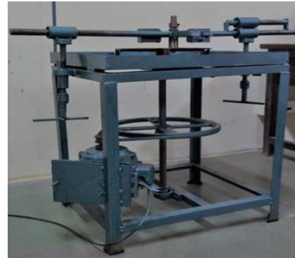
Fig. 16. Working prototype of the polishing machine
