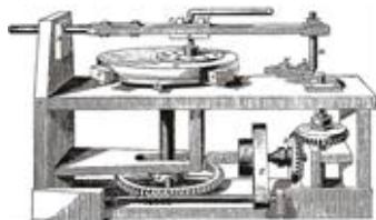
Fig. 4. Polishing machine by Henry Draper
