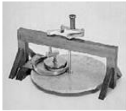
Fig. 2. 2nd Polishing machine by Leonardo da Vinci
