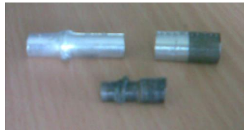
Figure 6.9: Specimens For Hardness Test. (Aluminum – Aluminum ,Aluminum – Mild Steel , And Mild Steel – Mild Steel )
