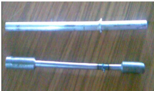
Fig.5: Welding of Similar metals
