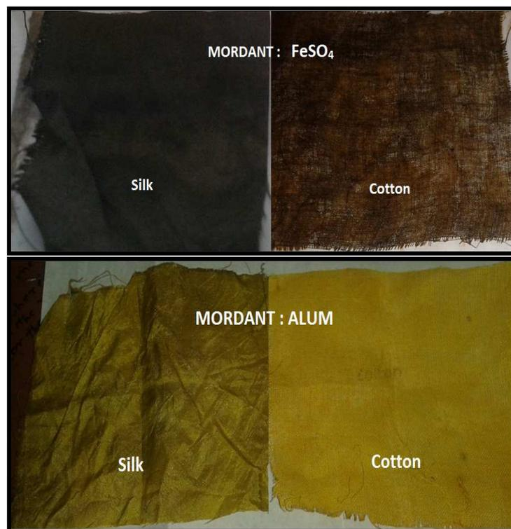
Fig 1: Cotton and silk cloth after dyeing in presence of mordant FeSO<sub>4</sub> and alum.
