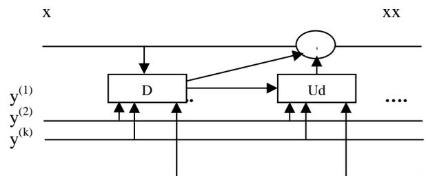
Figure 3.1. Adaptive update lifting scheme
