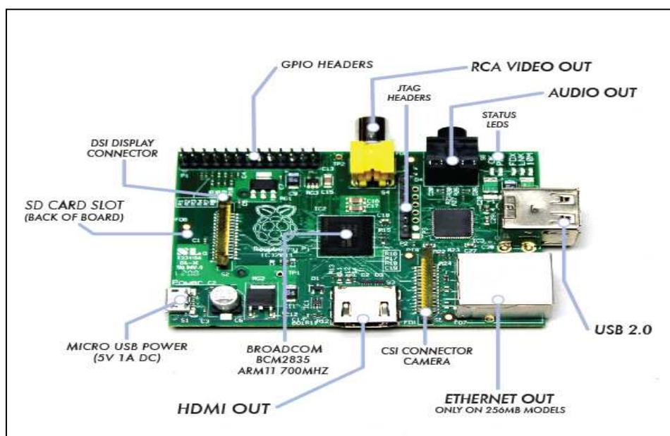
The Raspberry Pi is a low cost, credit-card sized computer that plugs into a computer monitor or TV, and uses a standard keyboard and mouse. It is a capable little device that enables people of all ages to explore computing, and to learn how to program in languages like Scratch and Python. It's capable of doing everything you'd expect a desktop computer to do, from browsing the internet and playing high-definition video, to making spreadsheets, word-processing, and playing games.
