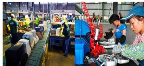
This sector is well organized as compared to Informal sector. It contain proper infrastructure, some technical staff to dismantle e-waste. It is a Combination of manual disassembly and refinery to upgrade materials limited reuse. This sector works with controlled detoxification and disposal environment, health and safety system as compared to informal sector.[4]
