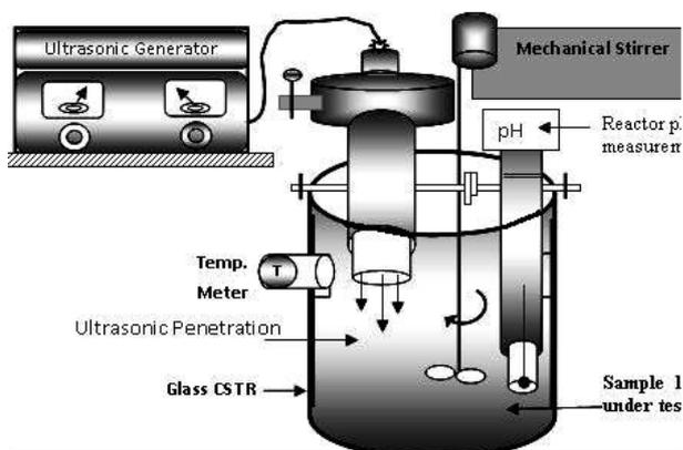
Fig.(1.1): Prototype laboratory Equipment for penetration of ultrasonic waves in the electrolyte solution
