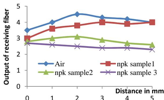
Figure 5 Optimization of distance between the sensor probe and reflector as 2 mm.
