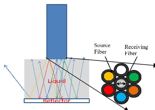
**Figure 2. Working principle of Optic fiber based NPK sensor**
