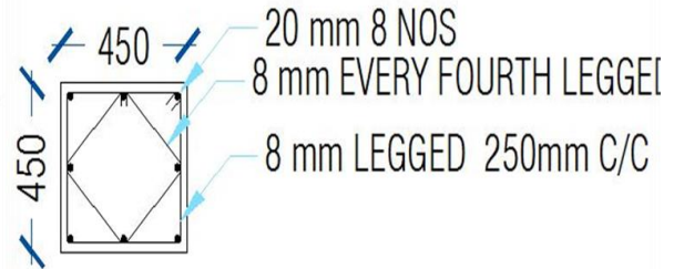
Fig No. 4.2.1 Detailing of Uniaxially loaded column
