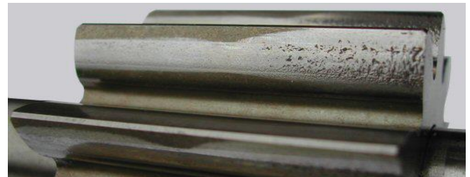
Fig.7 pitting (surface fatigue)
