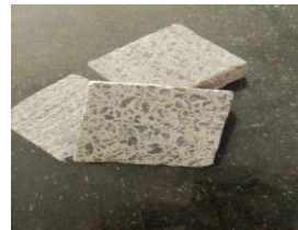
Fig.5 Sample Abrasion Result
