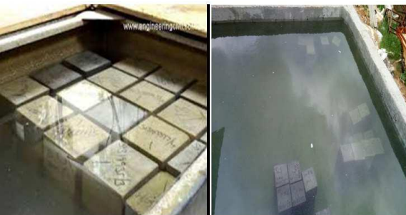
Curing of cubes and cylinders
