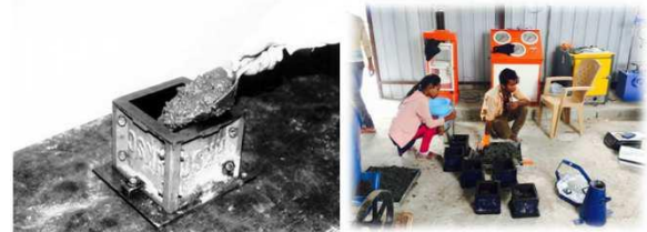
Filling the mould (for 150 mm cube 3 equal layers)
