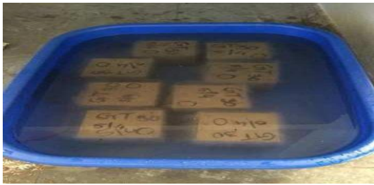
Fig.1 Shows specimens immersed in HCl solution
