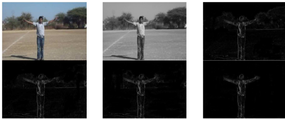
Figure 9: Image from database sequence, grayscale conversion, “Adaptive mixture models” [14], “Haritaoglu” [15]. “Romain” [16], and described technique. (Read row-wise).
