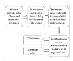
The GPS module with the help of antenna and satellite communication system measures the location coordinates in NMEA format and is converted when connected through USB, the virtual communication ports on computer allows to write program to process the data in readable format.
