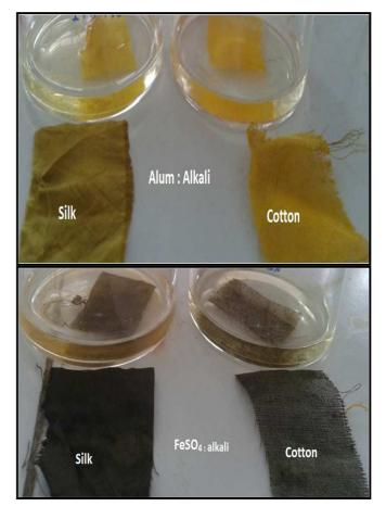
Fig 3: Cotton and Silk dye color faded in presence of alkali.
