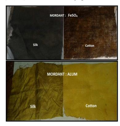
Fig 1: Cotton and silk cloth after dyeing in presence of mordant  $FeSO_4$  and alum.
