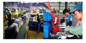
This sector is well organized as compared to Informal sector. It contain proper infrastructure, some technical staff to dismantle e-waste. It is a Combination of manual disassembly and refinery to upgrade materials limited reuse. This sector works with controlled detoxification and disposal environment, health and safety system as compared to informal sector.[4]
