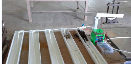
Fig.1. Photograph of s system used for drip irrigation system using moisture sensors.
